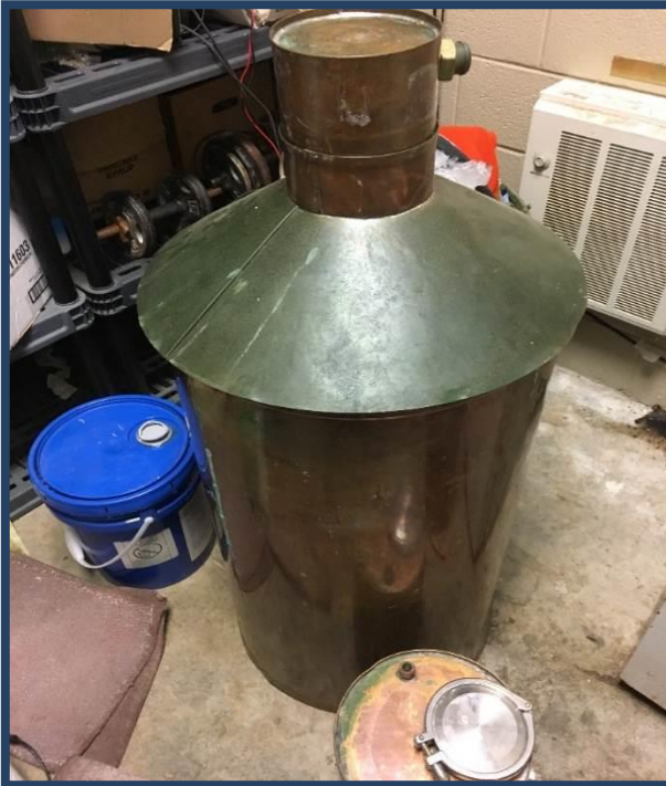
Still comprising of the Cap and Boiler
