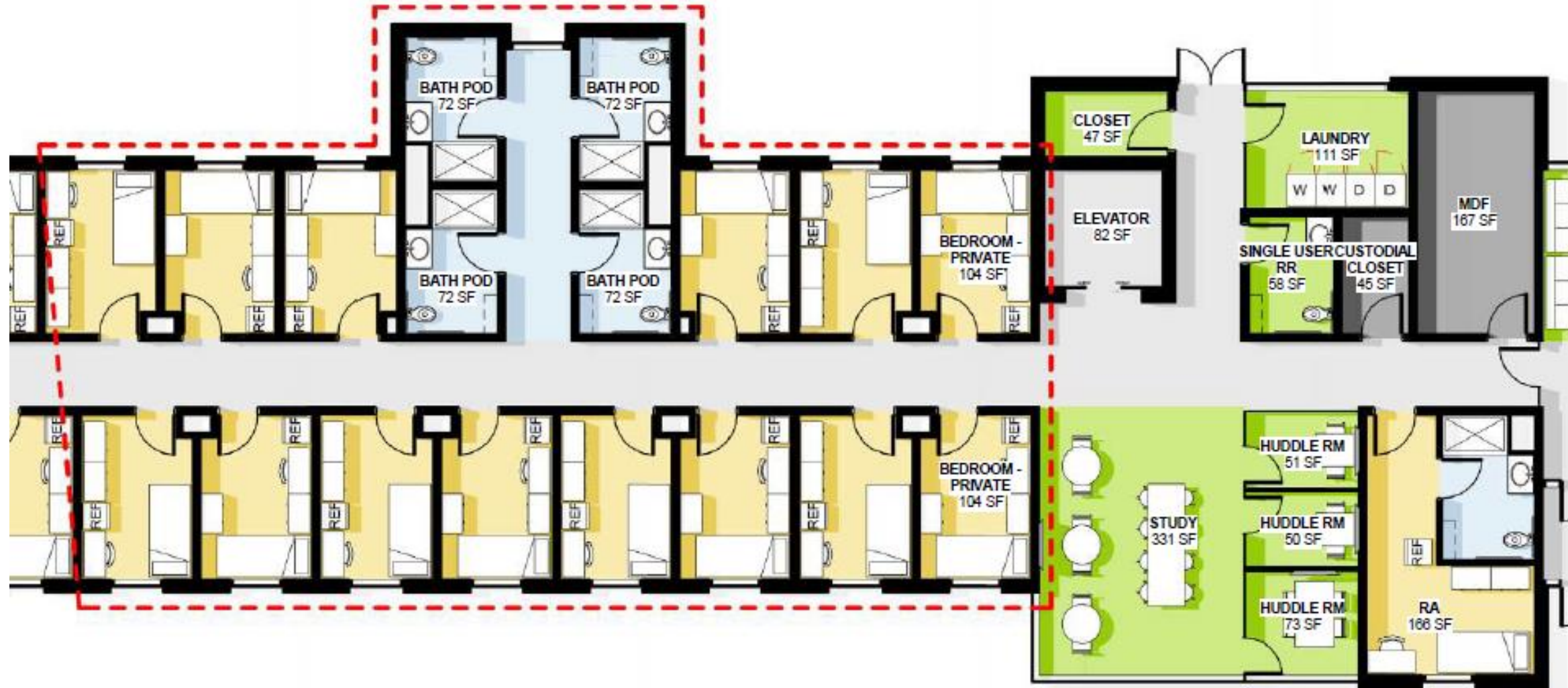
Typical Pod Configuration with adjacent Common Space
